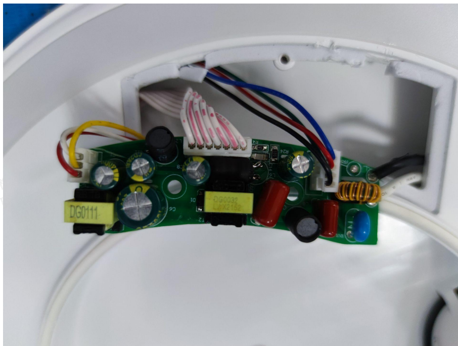
Photo 12 - LED driver 1 view of model RAVOLE2300C
