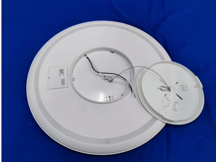
Photo 7 - Internal view of model RAVOLE2600C, also represents others
