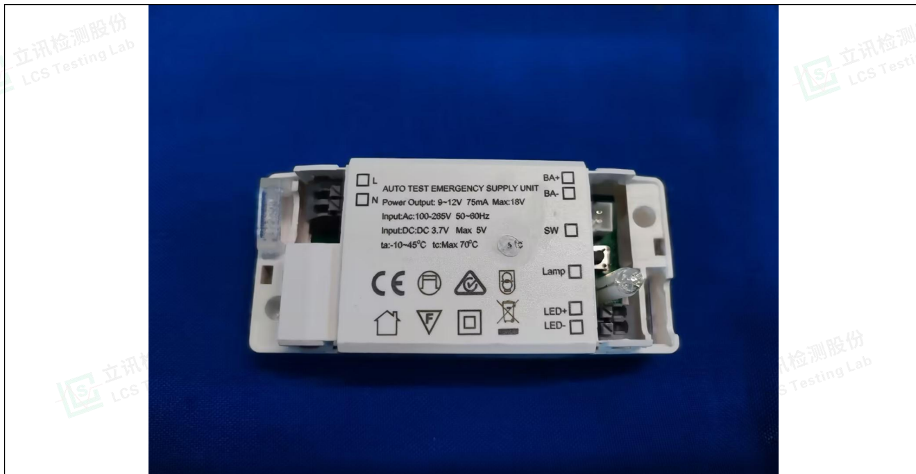
Photo 11(LED emergency driver)
