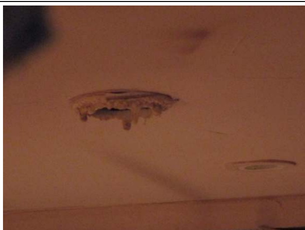
Photo 31: The exposed surface of the specimen after test duration of 3 minutes, showing the bezel of specimen 'D' fused.
