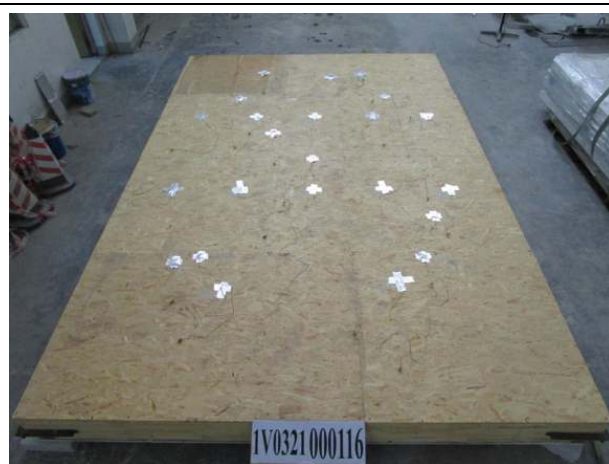
Photo 30: The unexposed surface of the specimen before the test.
