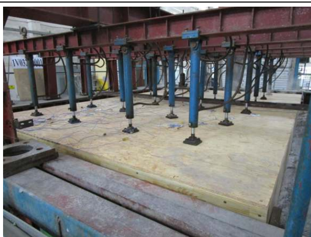
Photo 33: The unexposed surface of the specimen after test duration of 15 minutes.
