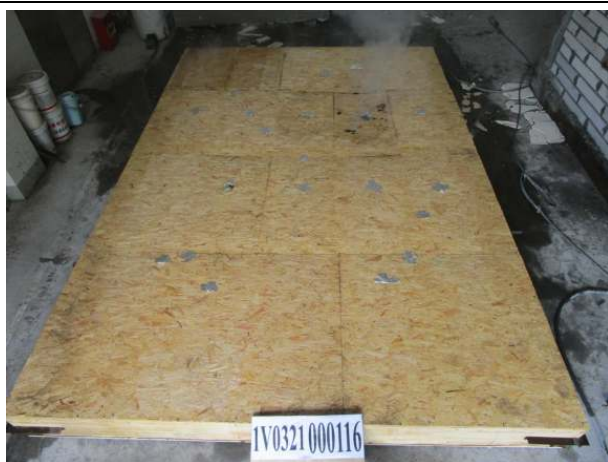
Photo 35: The unexposed surface of the specimen after the test.
