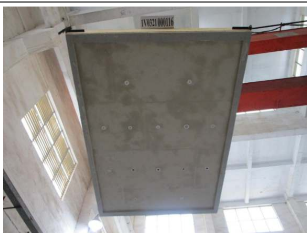
Photo 29: The exposed surface of the specimen before the test
