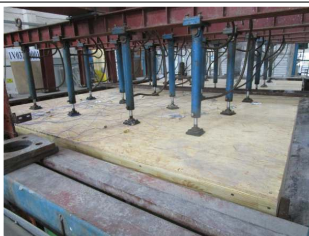
Photo 34: The unexposed surface of the specimen after test duration of 30 minutes.
